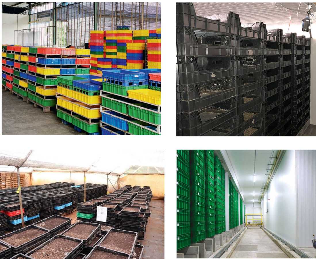
FIGURE 5: DIFFERENT DIMENSIONS AND SHAPES OF REARING CRATES AND STACKING METHODS. TOP LEFT: AERATION FRAMES BETWEEN LAYERS OF CONVERSION CRATES (EAWAG). TOP RIGHT: CRATES DIRECTLY STACKED OVER EACH OTHER (BETTER INSECT SOLUTIONS). BOTTOM LEFT: CONVERSION CRATES ARE STACKED CROSSWISE IN THE FACILITY OF INSECTIPRO, KENYA (DIENER/ECLOSE). BOTTOM RIGHT: RAILS USED FOR AUTOMATIC LOADING OF CRATES AT THE PROTIX FACILITY, NETHERLANDS (PROTIX).
