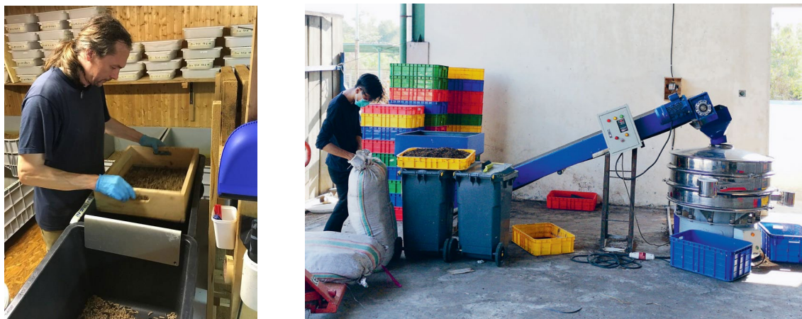
FIGURE 8: LEFT: MANUAL SEPARATION OF LARVAE AND FRASS (DIENER/ECLOSE). RIGHT: VIBRATING SIEVE TO SEPARATE LARVAE AND FRASS WITH BAGGING (EAWAG).
