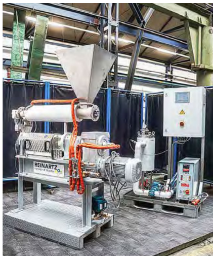
FIGURE 9: TOP LEFT: SMALL-SCALE PRESS FOR DEFATTING OF DRIED BSF LARVAE, PRODUCING PROTEIN MEAL (EAWAG). TOP RIGHT: FILLING OF DRYER WITH WET LARVAE (EAWAG). BOTTOM LEFT: LARGE-SCALE DEFATTING PRESS FOR REMOVING FAT FROM BSF LARVAE (REINARTZ). BOTTOM RIGHT: PELLETIZING AND PASTEURIZATION OF FRASS (BUEHLER GROUP).
